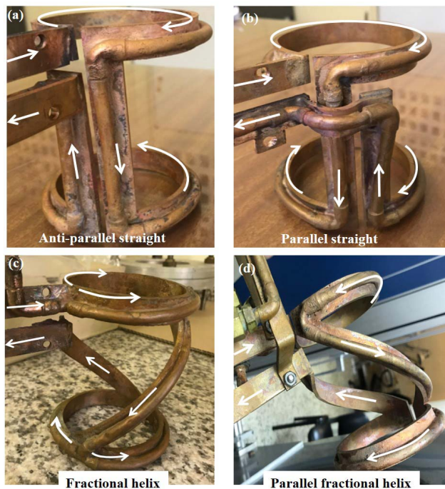
Fig. 2. (a)–(d) Pictures of the APS antenna, the PS antenna, the FH antenna, and the PFH antenna, respectively. The white arrows indicate the direction of the current at a given time. The two “horizontal” strips to the left of each antenna are dedicated to their connection to the matching network. One can see the copper tubes for water cooling soldered on the antennas.
