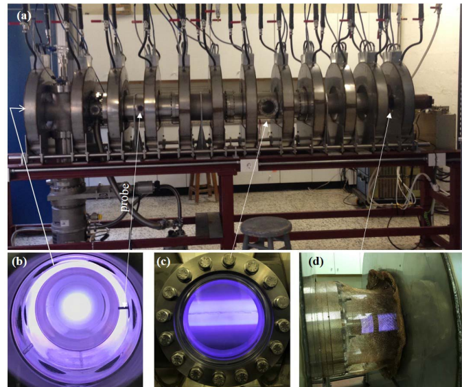
Fig. 1. (a) Picture of the Polaris linear plasma device where one can see the 12 magnets with their power cables and the water cooling connections. (c) RF antenna with the matching network. (d) Pumping system. Also is visible, the window ports where the images in (c) and (d) are taken. (b) Fused silica window that acts as an end-plate where the Langmuir probe can be seen.
