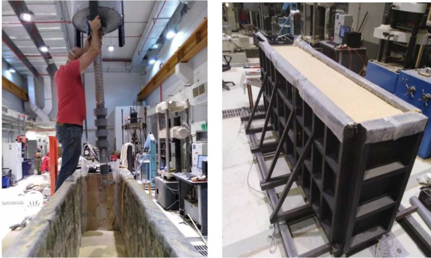
FIG. 8 Filling the soil retaining system with sand using pluviation.
