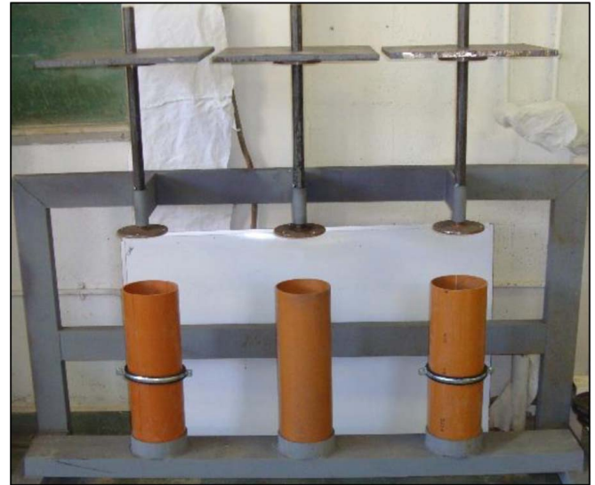
Fig. 6. Custom-fabricated 1D consolidometers.
