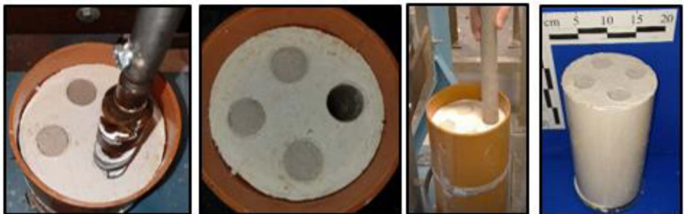
Fig. 9. Drilling holes in kaolin specimen and sand column installation.
