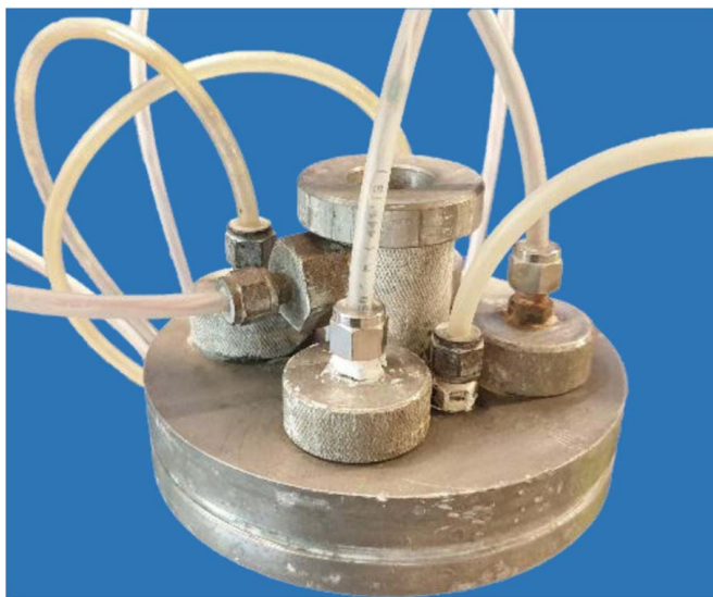
Fig. 3. Side view of the upper cap showing the fittings and tubing to completely isolate the cell pressurized water from leaking toward the sensors and the specimens.
