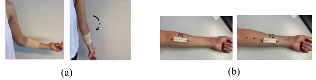
Fig. 9. The effect of (a) moving the arm and (b) changing the position of the flexible filter on the S-parameters response.
