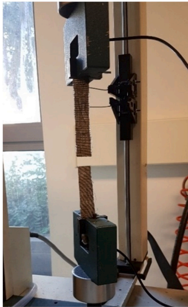
Fig. 2. Tensile test setup of hemp fabrics.
