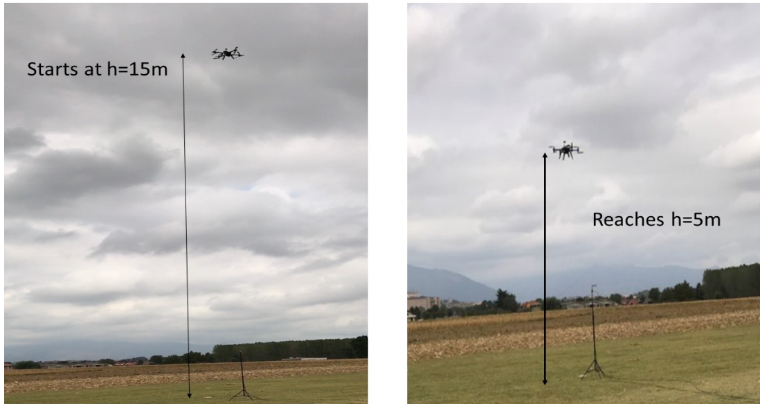
Figure 6.9: Vertical approach: Drone flying over the field starting at an altitude of 15m and reaching 5m.
