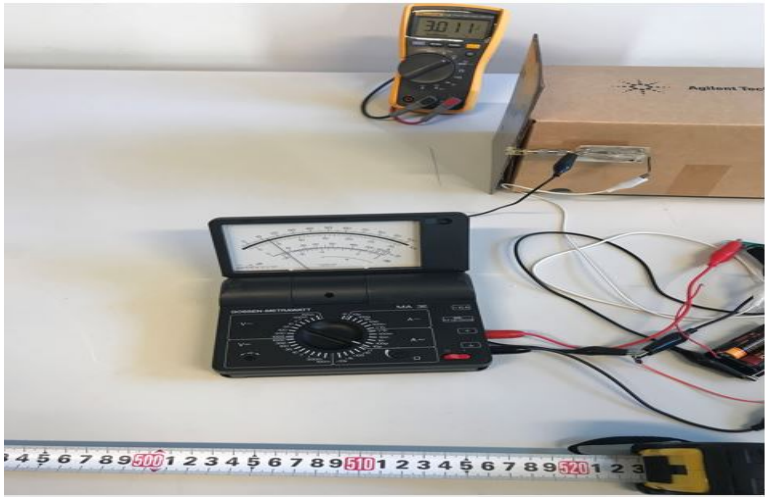
Figure 5.7: Measured distance and output voltage of the wake-up circuit design.
