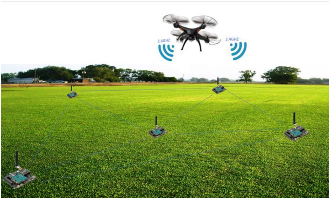
Figure 6.7: RF energy harvesting from the drone's telemetry signals.
