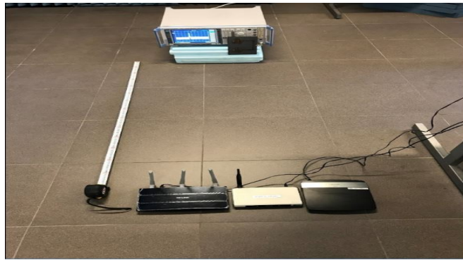
Figure 4.9: Experimental setup 2: Monitoring the Pr level from 3 APs placed next to each other.
