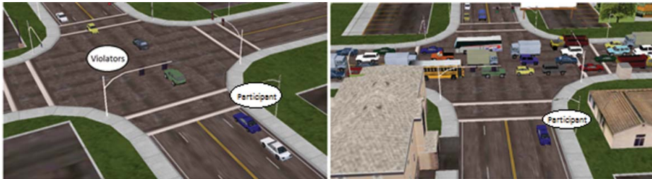
Figure 1. Schematics showing the red-light violations scenario (to the left) and the blocked intersection scenario (to the right) from the American University of Beirut driving simulator user interface (Danaf, Abou-Zeid, & Kaysi, 2013).
