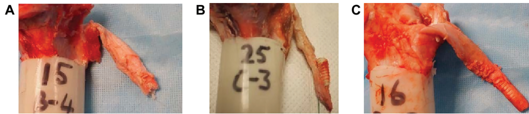
Figure 5. Modes of graft pullout failure observed. (A) Failure at graft bone plug-tendon interface. (B) Graft pullout with interference screw pullout. (C) Graft pullout without interference screw pullout.
